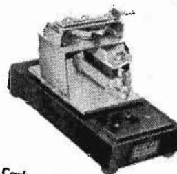
Carbon filling machines for precision filling of carbon microphones.
